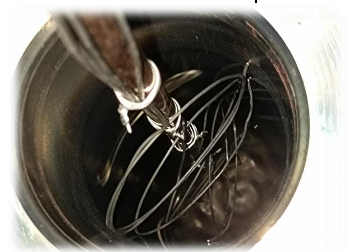
Inside wall thermocouples
